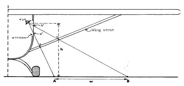
Figure 2 Schematic diagram of aircraft configuration for strip width sampling (Norton-Griffiths, 1978). W is marked out on the tarmac, and the two lines of sight a' – a – A and b' – b – B established. The dowels/streamers are attached to the struts at a and b. a' and b' are the window marks.
