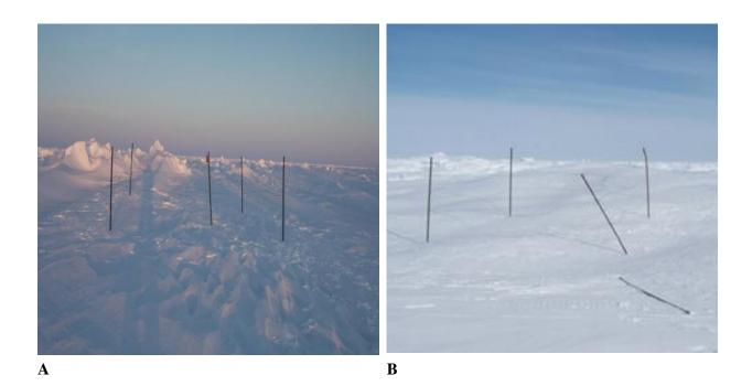
**Figure 3:** Polar bear sampling stations used in past work. The metal T-Bars are driven into the sea-ice and wrapped with 2 barbed wires with the lower one about 1.5ft off ground and the top one 1.5 ft from the lower one (Fig 3A). A sampling station following a polar bear sampling event (Fig 3B.)
