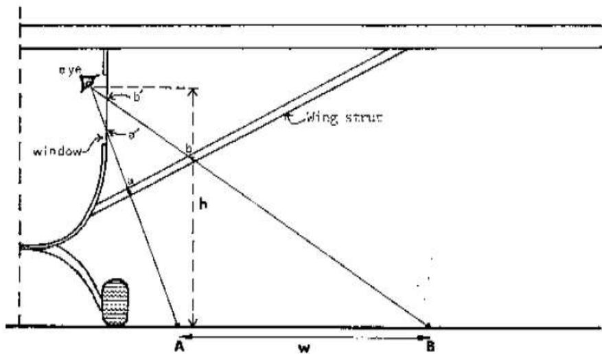
Figure 2: Schematic diagram of aircraft configuration for strip width sampling North-Griffiths (1978).  $w$  is marked out on the tarmac, and the two lines of sight  $a'-a$  and  $b'-b$  establish, whereas  $a'$  and  $b'$  are the window marks.
